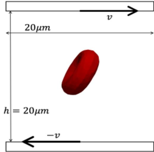
Figure 1. Simulation setting with indicated velocities of the fluid at the boundaries generating the uniform shear flow.
