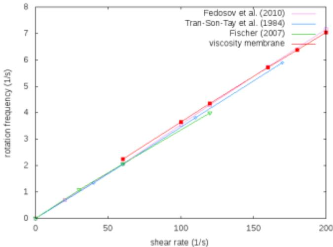
Figure 5. Rotation frequency for adjusted model including visco-elastic modulus (red line) and experimental data (other colors) taken from [6,7,14].
