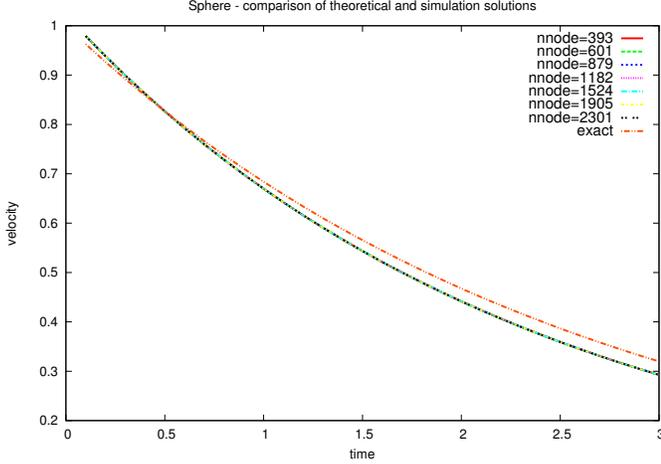
Fig. 2. Velocity profiles for different sphere triangulations are nearly identical and correspond well to the analytical solution, when the mass of IBPs is adjusted.
