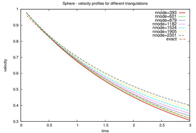
Fig. 1. Not adjusting the mass of immersed boundary points results in different velocity profiles for simulations that differ only by the number of triangulation nodes.
