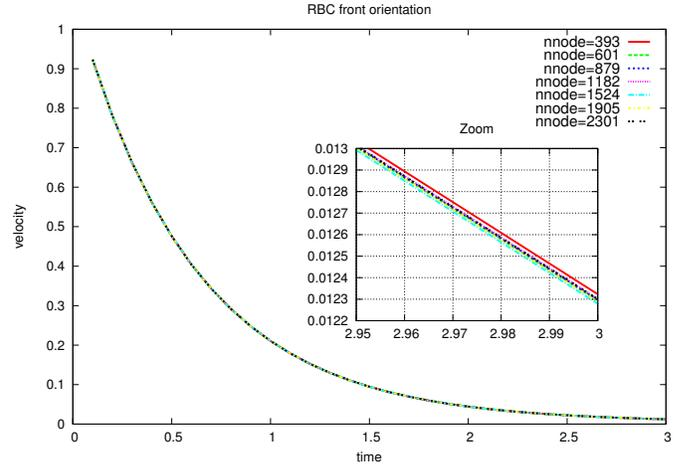
Fig. 4. Red blood cell with various surface triangulations was immersed in a stationary fluid "facing" the direction of its initial velocity. Mass of IBPs was properly adjusted. The velocity profiles are nearly identical. The relative error  $\frac{v_{393} - v_{2300}}{v_{2300}} = 0.19\%$  at the time  $t = 3$ .
