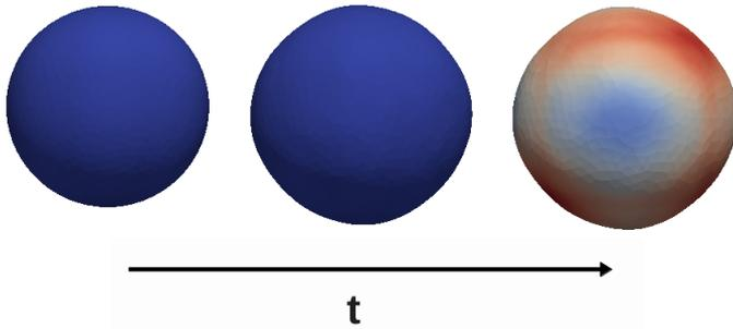
Fig. 3: Figures of spheres in experiment with length-normalized local area forces in three different time steps, from left to right. The colors correspond to magnitude of acting forces in each node from blue the smallest to red the largest. The figures were created in [7]
