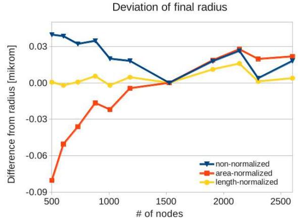
Fig. 2: Deviation of final radius for different number of mesh nodes, using area-normalized (red line, square symbols), length-normalized (yellow line, circle symbol) and non-normalized (blue line, triangle symbol) local area forces
