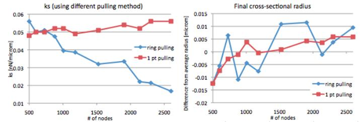
Fig. 7: Comparison of two stretching methods: On the left - fitted stretching coefficients, on the right - corresponding relaxed cross-sectional radii.
