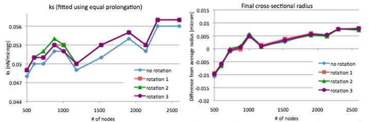
Fig. 5: Comparison of rotated meshes: On the left: stretching coefficient  $k_s$  fitted using the same force to achieve the same prolongation. On the right, corresponding relaxed cross-sectional radii.
