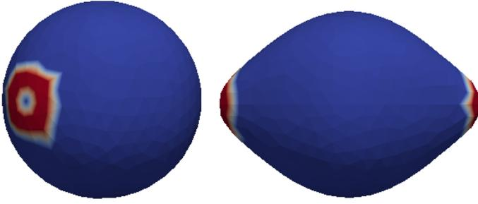
Fig. 6: A sphere that is stretched by applying forces along two rings.  $t = 0$  on the left, on the right the sphere is after relaxation. The displayed mesh has 601 surface nodes.
